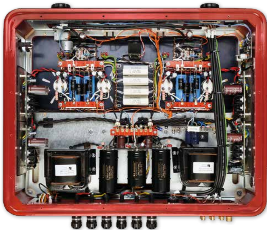
RIGHT: Inside the Rhapsody revealing the point-to-point wiring, partly with vdH cable, custom output transformers [bottom, left/right], Mundorf Mlytic PSU capacitors [bottom] and separate L/R PSU regulation [far left/right]
